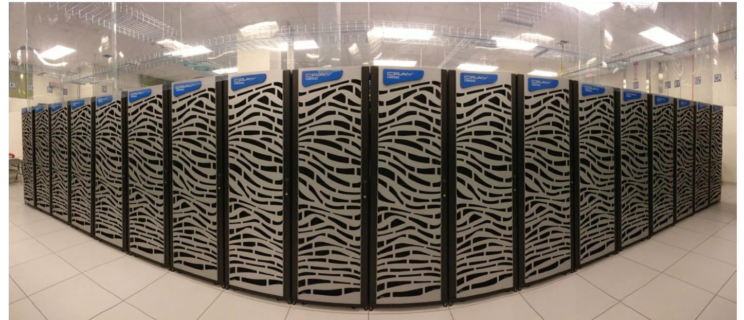
The NOAA Hera supercomputer located in Fairmont, WV. Hera has 52,640 Skylake processors with multiple grey cabinets (20 are shown in the image) and is labeled with CRAY CS500. The racks of hardware components are stacked vertically to save space, allow for ease of connecting the many nodes and cores of the supercomputer, and improve efficiency in cooling.
