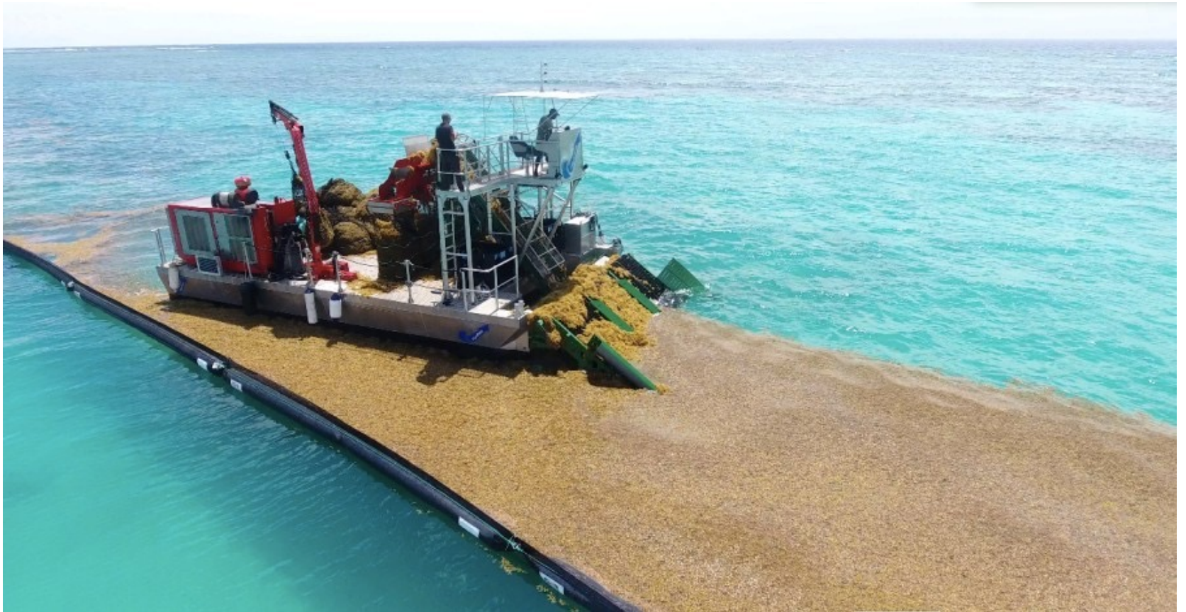
AlgaeNova harvesting equipment that operates on the water.
