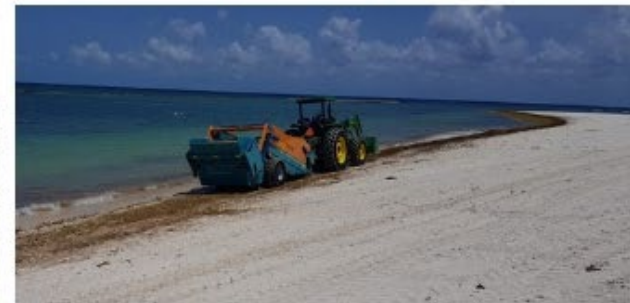
Scarbat (Beach Trotters) machine, a beach cleaner used by some hotels
