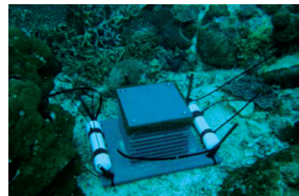
An Autonomous Reef Monitoring Structure (ARMS), like the one shown, is designed to mimic the reef environment and attract colonizing coral reef organisms.
