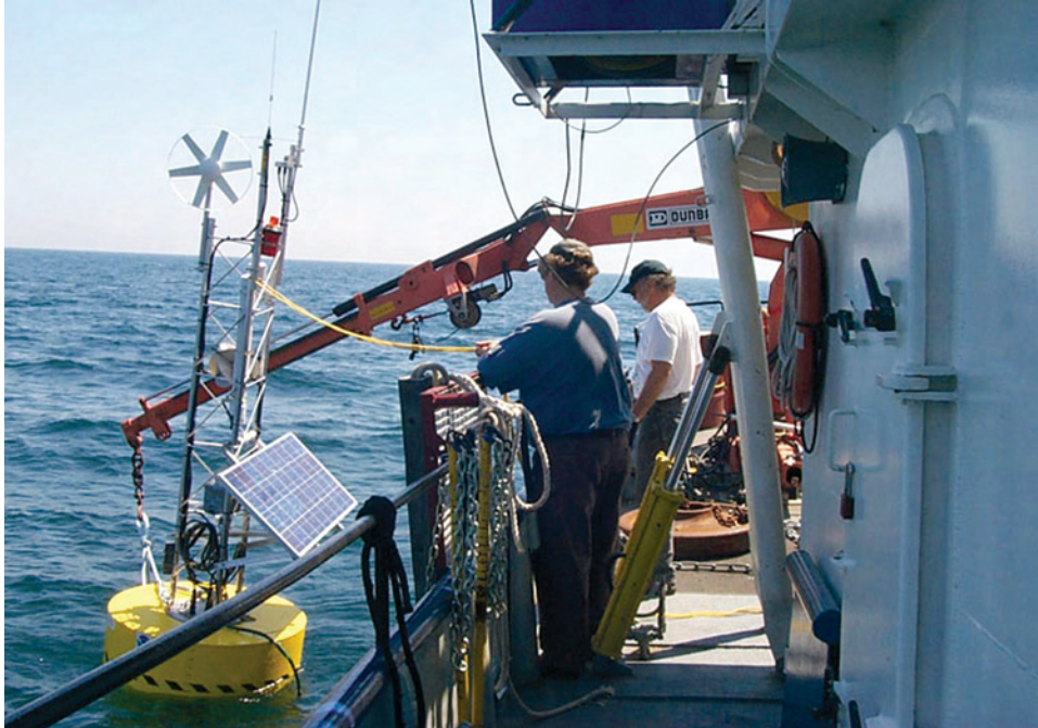
Installing a RECON (Real-time Environmental Coastal observations Network) buoy, a wireless Internet observation system that collects meteorological data and provides sub-surface measurements of chemical, biological, and physical parameters
