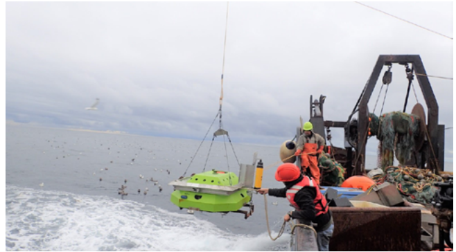
Staff deploy an innovative seafloor-mounted upward-looking echosounder (SME) technology to quantify the directional movements of fish over extended periods as part of the Year-Round Monitoring of Pollock Movements in Eastern Bering Sea.
