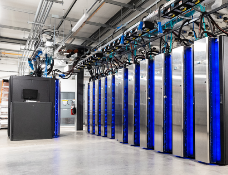
Twin supercomputers Dogwood (pictured here) and Cactus are the newest additions to NOAA’s weather and climate operational supercomputing system. Each operates at a speed of 12.1 petaflops, three times faster than NOAA’s former system. Credit: General Dynamics Information Technology
