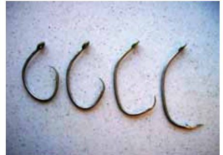
An example of the weak hook designed to reduce bluefin tuna bycatch.
