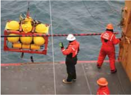
Scientists from the Office of Coast Survey and the University of New Hampshire lower a sophisticated echo sounder into the water to create a three-dimensional map of the sea floor. The data collected will help scientists better understand the underwater landscape and improve climate and ocean current circulation models.
