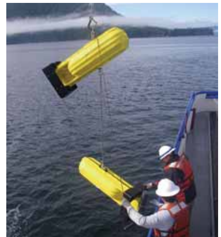
The Center for Operational Oceanographic Products and Services (COOPS) conducts surveys of tidal currents in response to user requests. Here, scientists deploy current meter buoys and anchors used for the surveys.
