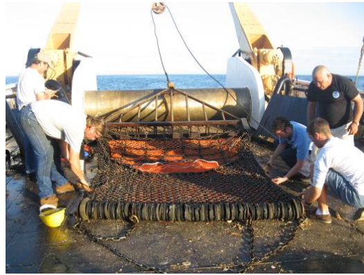
This standard dredge is 19 ft. in length, has an 8-ft. wide opening, & weighs about 1600 lbs. A sweep chain of heavy metal covers the opening & holds the dredge open. What could you catch?
