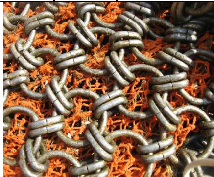
Rings (2 inch in diameter) & links cover the entire dredge. These rings on the dredge move across the bottom of the ocean floor collecting organisms. The net liner keeps fish & scallops in the dredge. It is build to withstand the impact of rocks. Notice the circle rings & double links.
