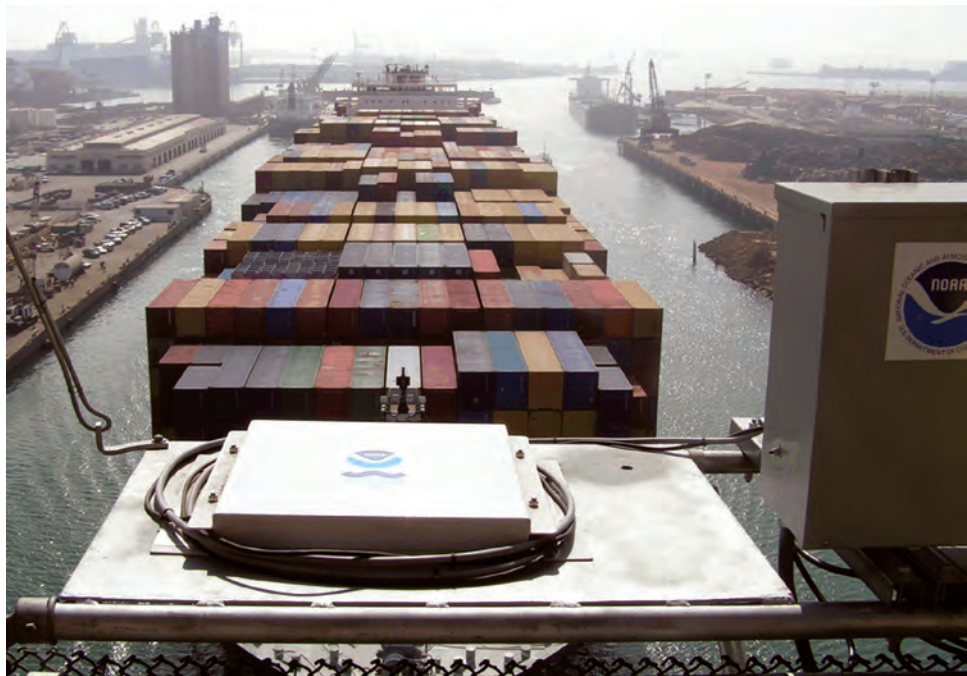
An air gap (bridge clearance) sensor, an integral part of PORTS®, installed on the Gerald Desmond Bridge, in Long Beach, California, helps ships determine proper clearance underneath the bridge
