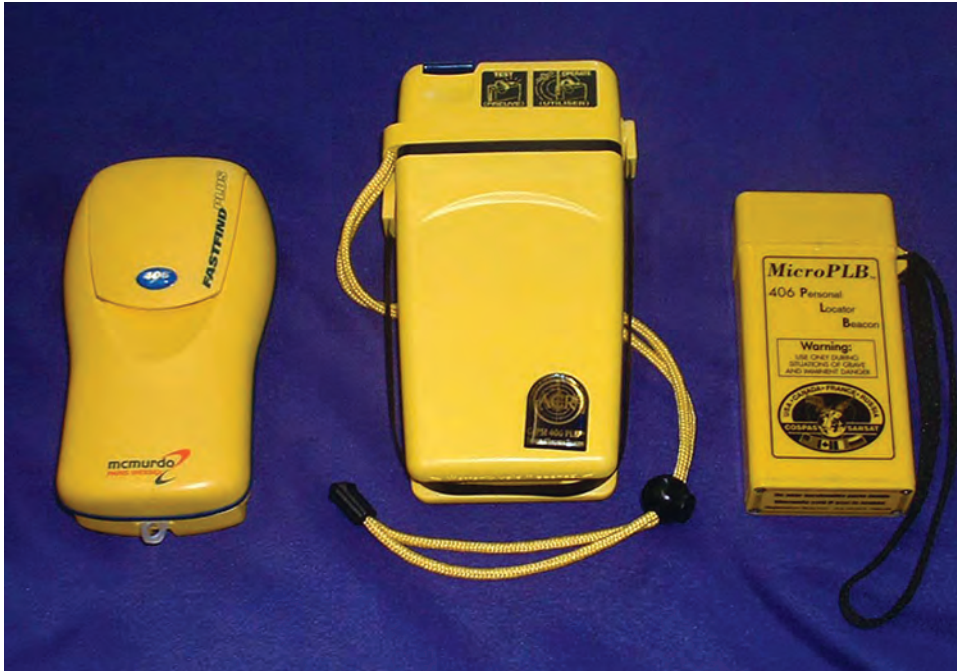
Emergency Position Indicating Radio Beacons (EPIRBs) and Personal Locator Beacons (PLBs), tracking transmitters which aid in the detection and location of boats, aircraft, and people in distress, interface with COSPAS-SARSAT
