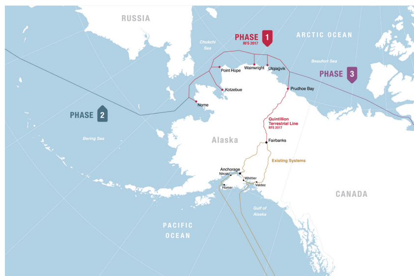
Construction is complete on the first phase of the Quintillion subsea and terrestrial fiber optic network, which extends over Alaska's North Slope and inland to Fairbanks. Map courtesy of Quintillion.
