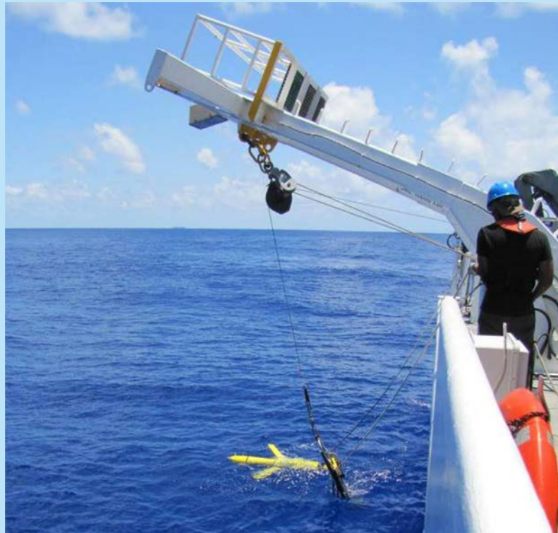
Figure 3.1. An unmanned underwater vehicle is deployed from a Naval Oceanographic Office (NAVOCEANO) survey vessel. (Image courtesy of U.S. Navy)
