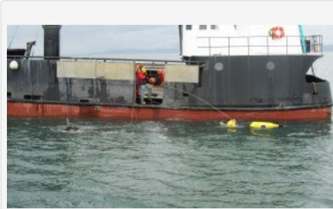
NOAA staff deploy a current meter off the Homer Spit.
