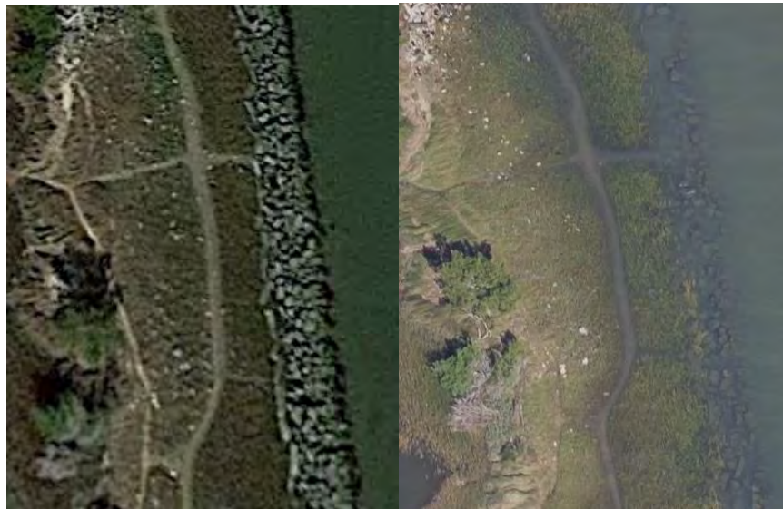
Figure 29. Charleston Harbor marsh system example at various tide levels, protected by armor stone (images courtesy of Google Earth and Bing Maps)
