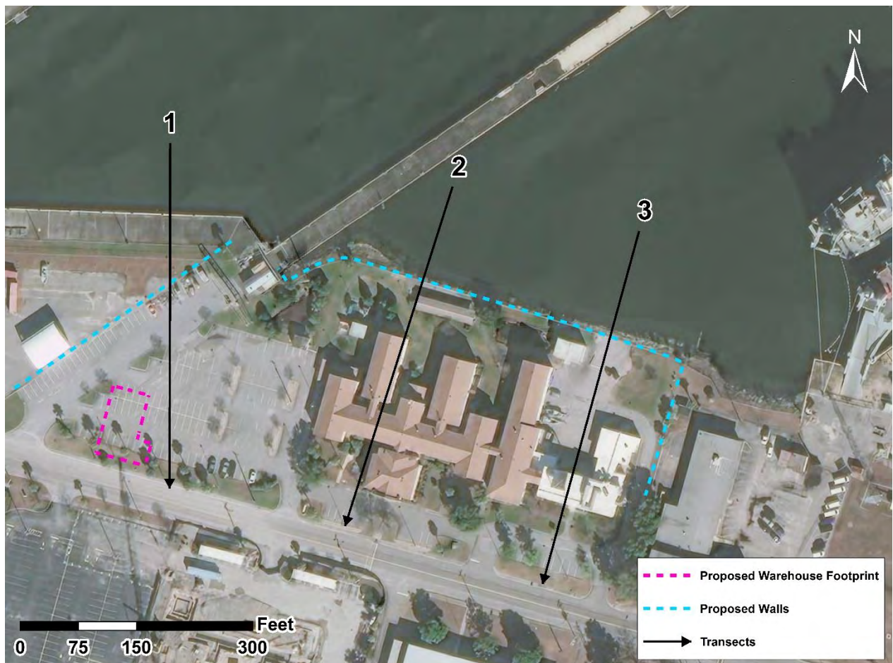
Figure 14. Transect layout for WHAFIS modeling of existing conditions and proposed wall conditions
