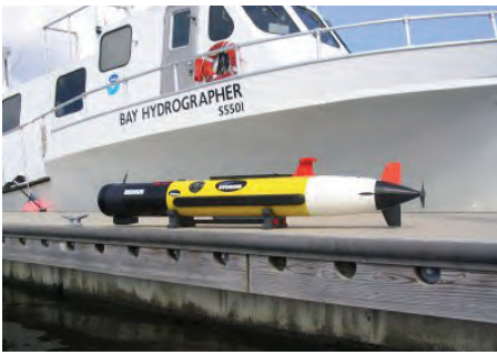
Autonomous Underwater Vehicles (AUV), also known as unmanned underwater vehicles, can be used to perform underwater survey missions such as detecting and mapping submerged wrecks, rocks, and obstructions that pose a hazard to navigation for commercial and recreational vessels. AUV and NOAA's Bay Hydrographer in Chesapeake Bay shown here.
