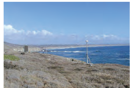
Representation of a HF radar system, known as CODAR. The CODAR ocean sensor is used to measure the speed and direction of surface currents.
