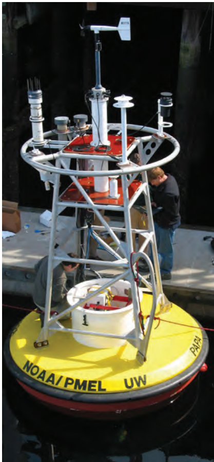
"Papa" NOAA buoys measure parameters such as air and sea surface temperature, wind, relative humidity, rain rate, and ocean currents and transmit this data via satellite communications multiple times daily in real time to meteorological and science centers for use in weather forecasting and climate study.
