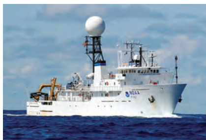
Dedicated solely to exploration, the ship conducts operations around the globe, mapping the seafloor and characterizing largely unknown areas of the ocean. Interesting seafloor features can be discovered with the deep water multibeam sonar mapping system. Sites are further explored with a Conductivity Temperature and Depth sensor (CTD) and a Remotely Operated Vehicle (ROV). Images and high-definition video from the underwater vehicles can then be sent from the vehicle to the ship to the shore all in real-time. This technology is referred to as "telepresence."
