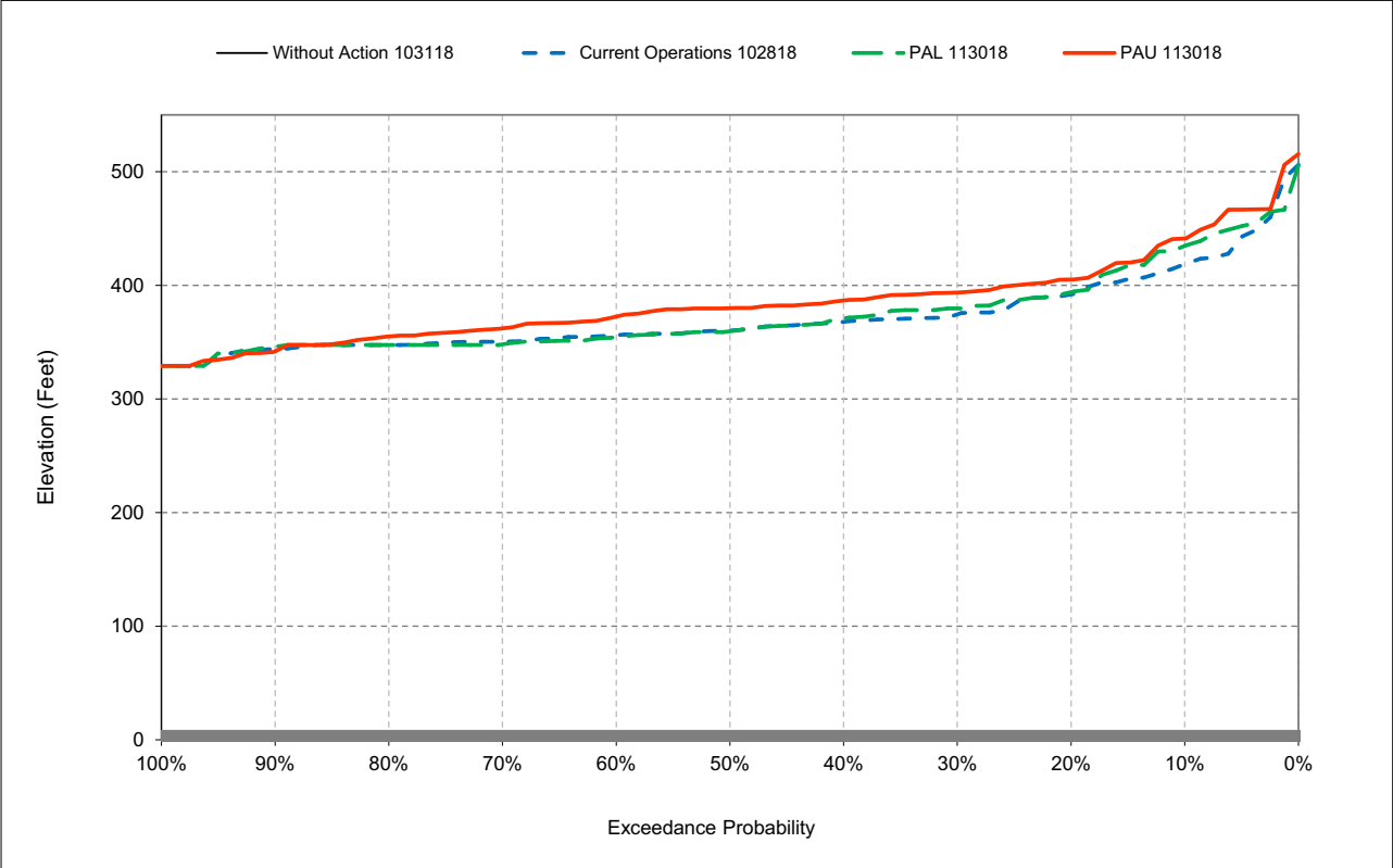
Figure 6a-2. San Luis Reservoir (SWP and CVP), Reservoir Pool Elevation, September
