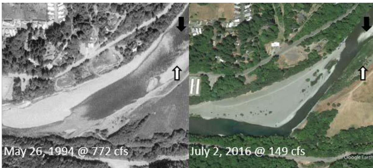
Figure 1. Changes at Social Security Bar on the Chetco River between 1994 and 2016. Filled arrows indicate new gravel bar, open arrows indicate improved vegetation (Google Earth 2018).
