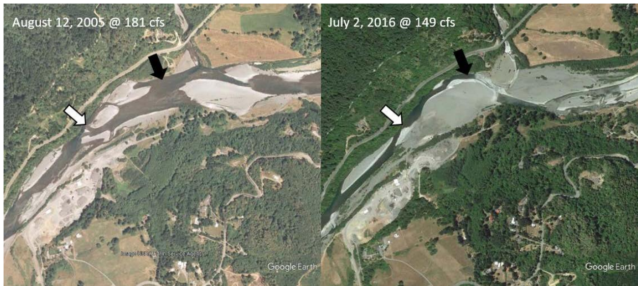
Figure 3. Changes at Freeman extraction location on the Chetco River at the Confluence of North Fork Chetco River between 2005 and 2016. Filled arrows indicate a narrowing low flow channel, open arrows indicate conversion of braided channels to a single one (Google Earth 2018).
