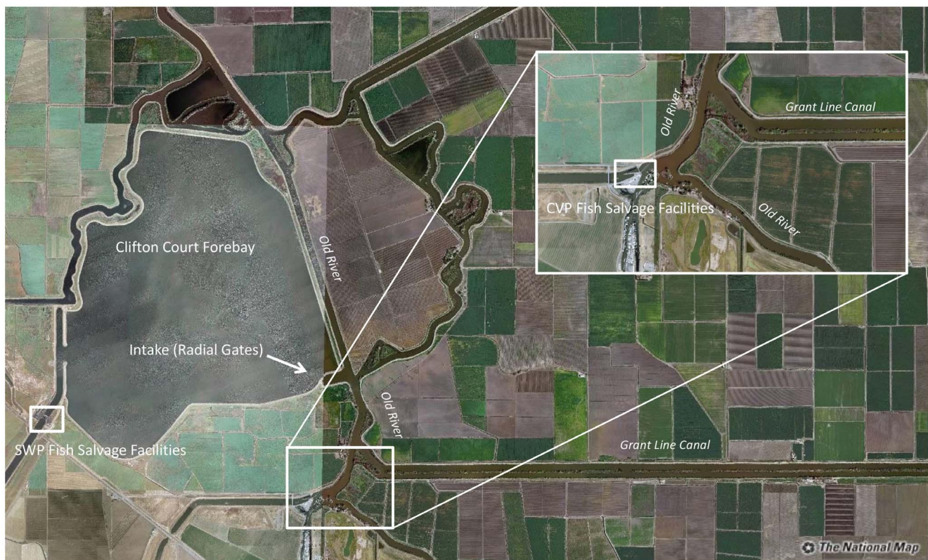
Figure 2. Aerial view of the layout of the two water diversion and fish salvage facilities. The State Water Project (SWP) diverts from Clifton Court Forebay that is filled from radial gates located on Old River; a distributary of the San Joaquin River. The Central Valley Project (CVP) diverts water directly from Old River. Image was downloaded from The National Map: http://nationalmap.gov/ . doi:10.1371/journal.pone.0101479.g002
