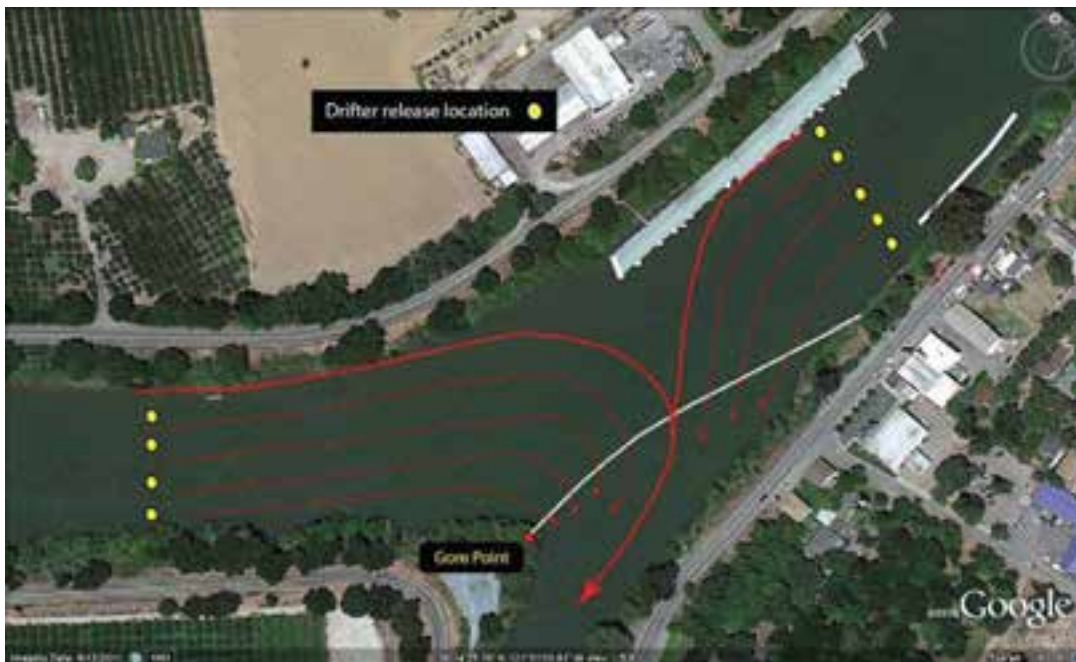
Figure B.4-6. Drifter Release Locations (yellow dots) During a Converging Stage and Modeled Particle Paths and Critical Streakline Under Converging Conditions
