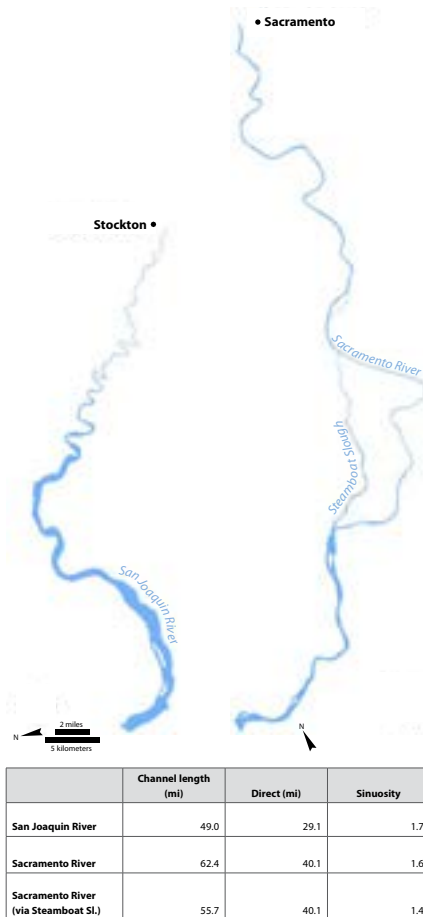
Figure 4.6. The San Joaquin and Sacramento rivers differ in width and sinuosity. Close to the Delta mouth, the San Joaquin is almost double the width of the Sacramento River. Moving upstream along both channels, the San Joaquin becomes a very sinuous with tight bends and much narrower tidal channel, while the Sacramento bends are much wider, reflecting greater riverine influence.
