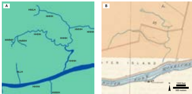
Figure 2.3. Assignment of certainty levels to channels. A channel network (A) off the Mokelumne River within lower Staten Island is shown with certainty levels (in order of interpretation, size, location, and tidal status) assigned to parts depending on sources used to map the network. One of the sources used to map the network, the early 1900s USGS topographic maps, is shown in (B), where not all historical channels are shown, due to reclamation. (B: USGS 1909-1918)
