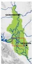
Figure 4.16. Connecting historically disconnected channels. This map illustrates how the historical channel network (in blue) has been linked up by cross-channels and meander cuts (yellow highlighted areas of the modern channel network, in gray). The cross-channels were created in the process of building cross-levees and established many of the Delta's "tracts," such as Frank's Tract and Drexler Tract. This increased connectivity has altered the routing of tidal water by making travel distances shorter, by and large, between given points.
