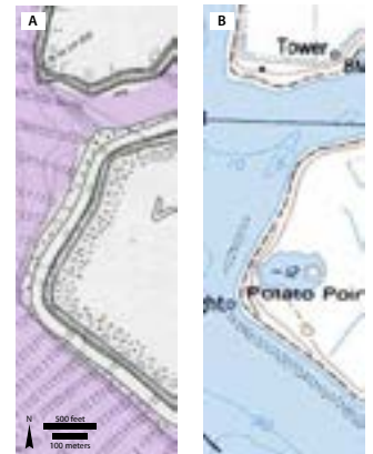
Figure 2.5. Historical channel width mapped based on remnant in-channel islands that outline the pre-reclamation edge of wetlands. The transparent light purple overlay in (A) shows the historical mapping on top of a 1908 Debris Commission map. The artificial levees (with a ditch and then a strip of wetland running along the channel edge) are now the edge of islands, as seen in (B). (A: Wadsworth 1908b, courtesy of the California State Lands Commission; B: USGS 1998)
