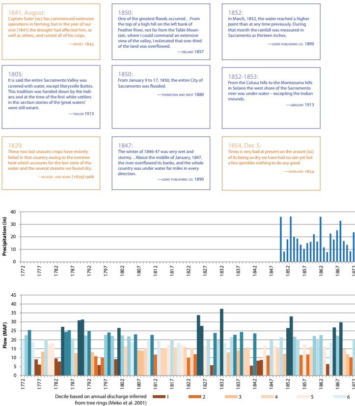
Figure 1.6. Wet and dry years of the recent past. This diagram was created from reconstructed Sacramento River runoff in million acre-feet (MAF), based on tree ring analysis by Meko et al. (2001). The bars showing the runoff magnitude are color-coded by the decile within which they fall, with the drier years represented in warm colors and the wetter in cool. The blue solid line shows unimpaired flow as reconstructed by the Department of Water Resources (2007) from the period of record (beginning in 1921). Immediately above the graph is precipitation at Sacramento
