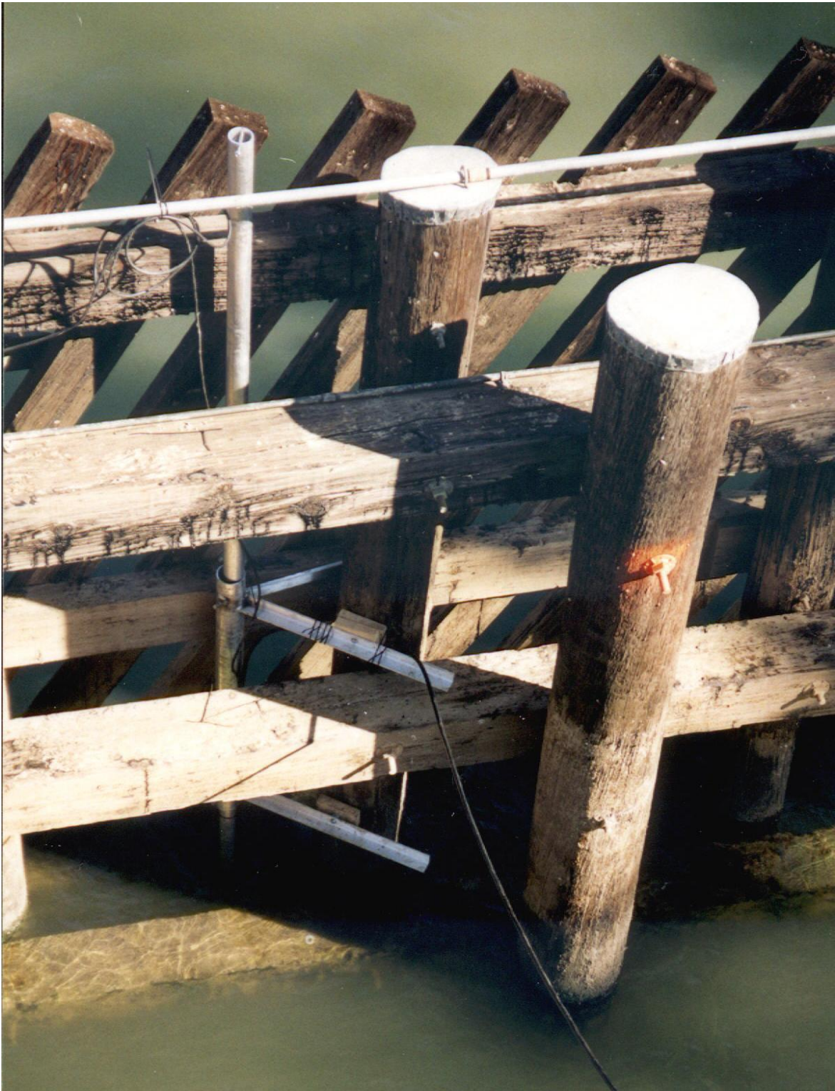
Figure 7. Typical mounting design for acoustic unit.
