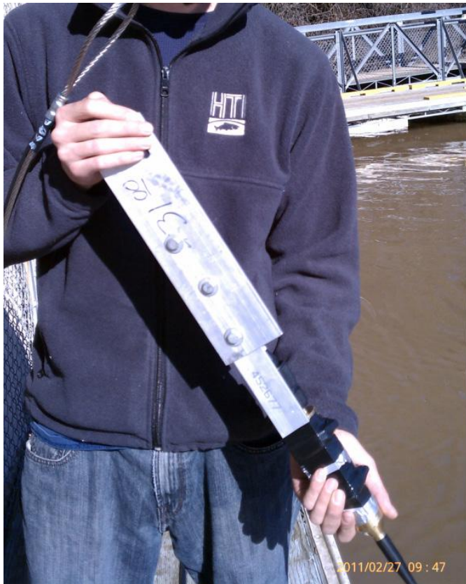
Figure 14. Example of the “Dock” mount used for the Hydrophones H1, and H6 at the GSNPB, 2011.
