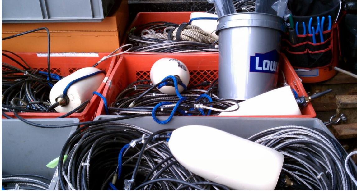
Figure 11. Hydrophone cables ready for deployment.
