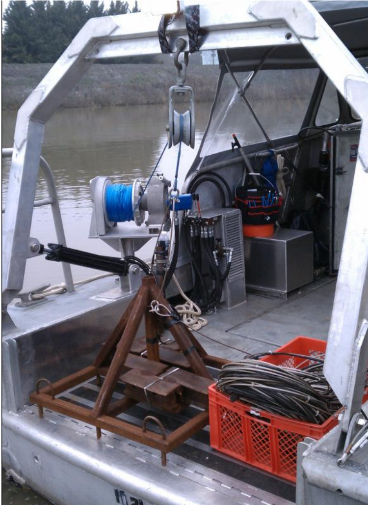
Figure 13. Example of the "Tower" mount used for deployment of hydrophones H3, H5, H8, H10, H12, H16, H18 and H20 at the GSNPB, 2011.
