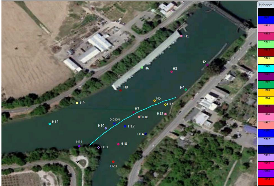
Figure 10. Location of hydrophones as deployed at Georgiana Slough NPB 2011.
