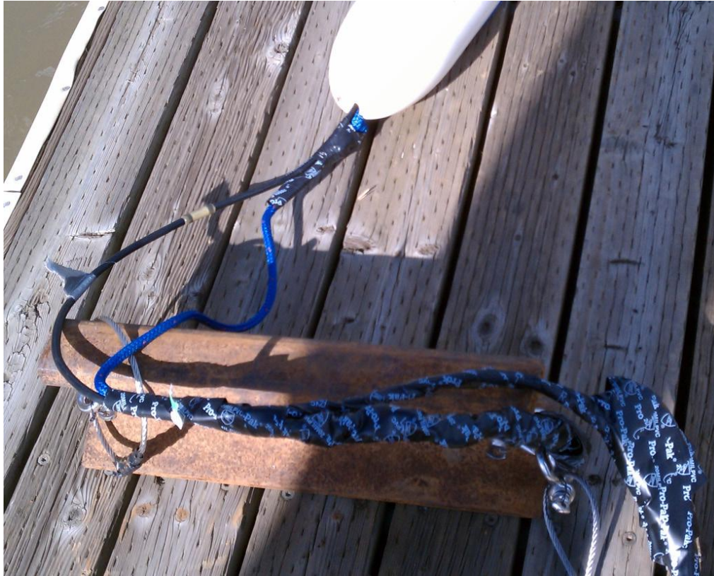
Figure 15. Example of the modified railroad tie mounts used for the at the autonomous data logger sites upstream and downstream of the main hydrophone array at the GSNPB, 2011.
