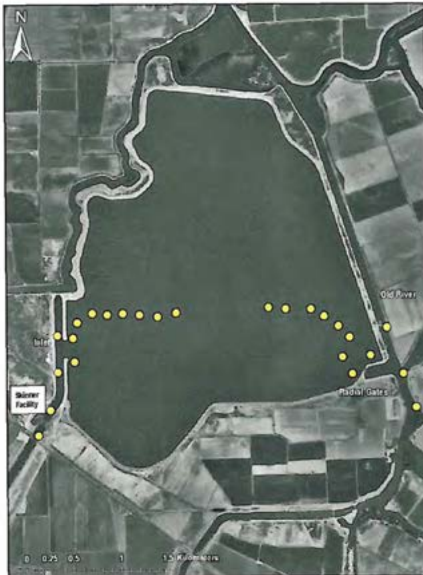
Figure 18. Fixed station receiver (29 total) locations within Clifton Court Forebay and Old River during the 2005 pilot study. The four receivers located within the SFPF are not shown. Locations of the receivers are indicated by yellow circles.
