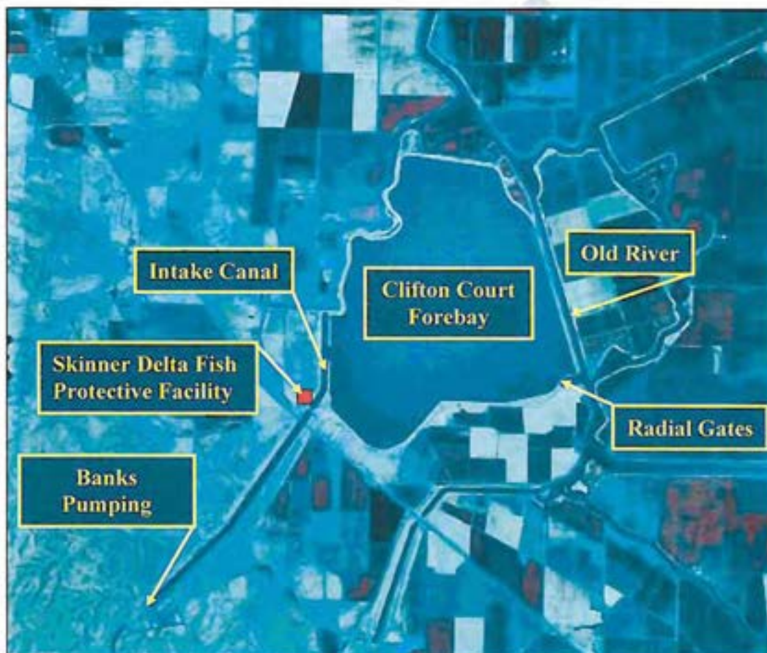
Figure 2. Aerial photograph of Clifton Court Forebay with the locations of Old River, radial gates, intake canal, Banks Pumping Plant, and the John E. Skinner Delta Fish Protective Facility. (National High Altitude Photography courtesy of the United States Geological Survey)
