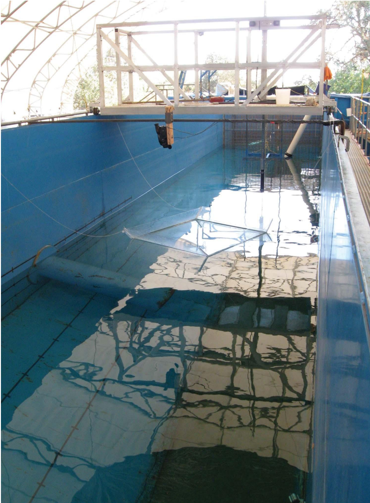
FIGURE 2. Top-view photograph of the fish-swimming flume, taken during fish acclimation under still water conditions. The water diversion pipe is visible below the overhead camera, and the fish-releasing cage is submerged at the upstream end of the flume. [Figure available online in color.]
