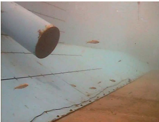
FIGURE 3. Underwater view of the flume taken by camera number 2, showing the water diversion pipe inlet and swimming juvenile Chinook Salmon. [Figure available online in color.]
