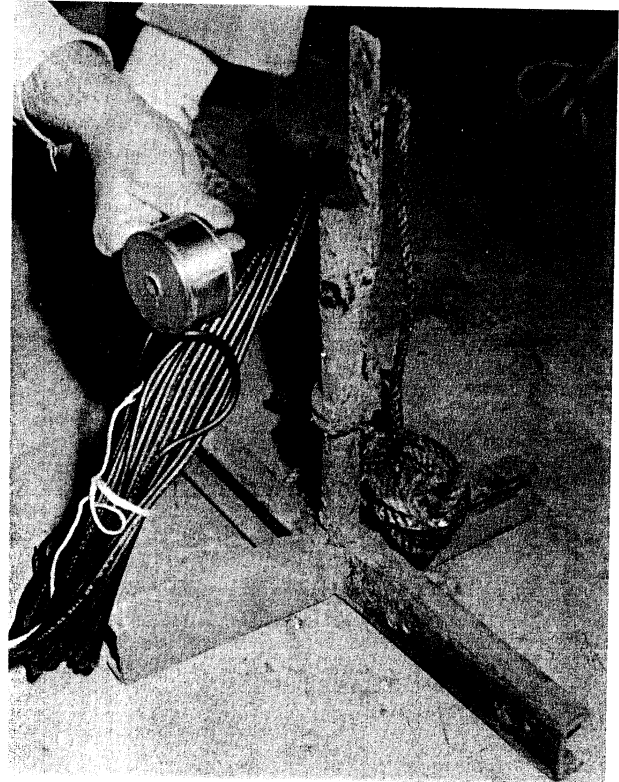
FIGURE 11. Hydrophone, iron stand used to hold it above the river bottom and lead-in cable. Photograph by Wm. F. Van Woert.
