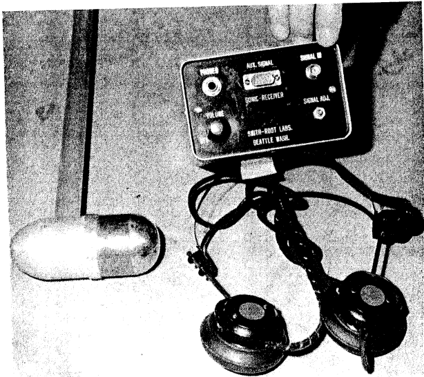
FIGURE 8. Portable probe (or hydrophone) and receiver for tracking sonic tags. Photograph by John A. Shaver.
