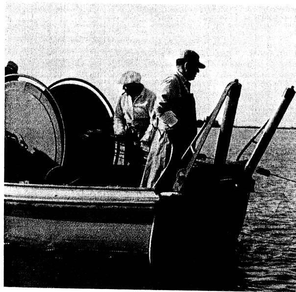
FIGURE 14. Trammel net being wound onto powered net reel on the M.V. Striper , San Joaquin River at Prisoners Point; fall, 1965. Photograph by Richard J. Hallock.
