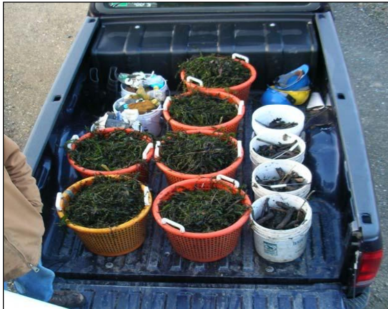
Figure 11- View of a 4X debris load ready for insertion into the release truck.
