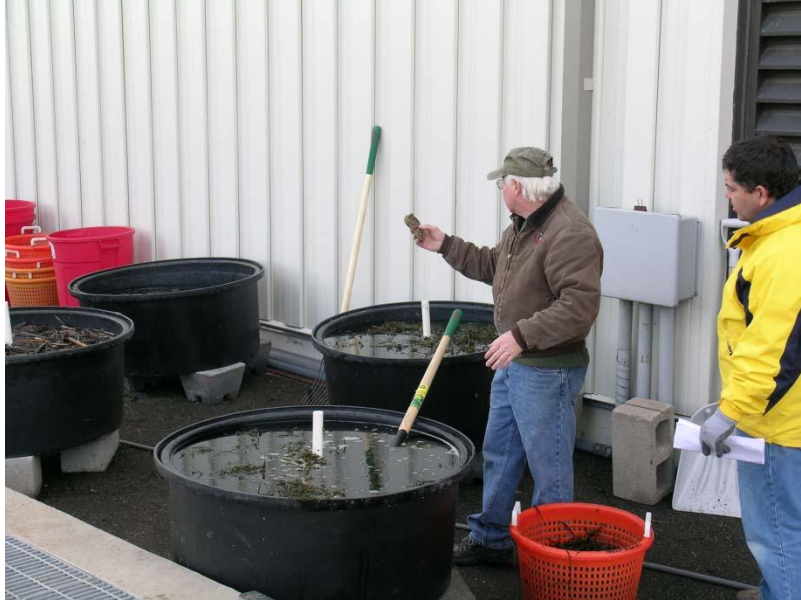
Figure 10- The three types of debris were kept submerged in individual 341-L (90-gal) containers.
