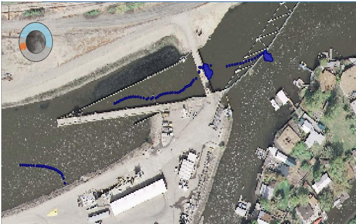
Figure 8. Example of secondary louver loss of a Chinook salmon (fish was released during high flow experiment and passed through the secondary louver not during a cleaning event).
