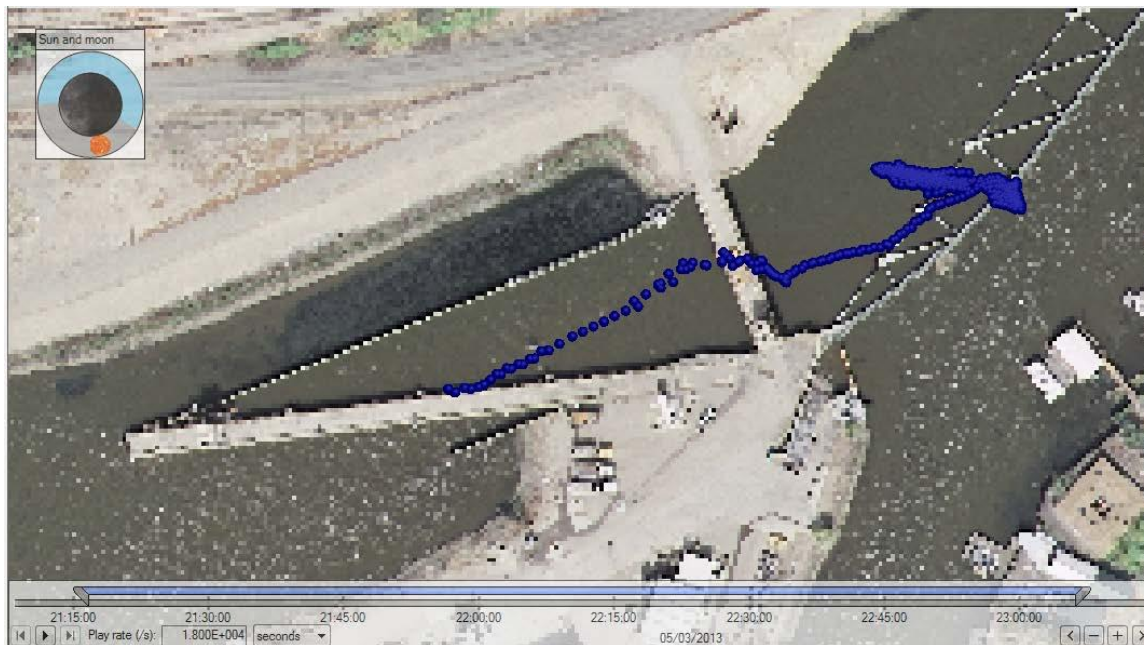
Figure C-13. Track of Chinook salmon 3967 (released at intermediate flow, total time in system was about 8 min: 4 min in the upstream channel, 1.7 min in the primary channel, and 2.8 min in the bypass pipes/secondary channel).
