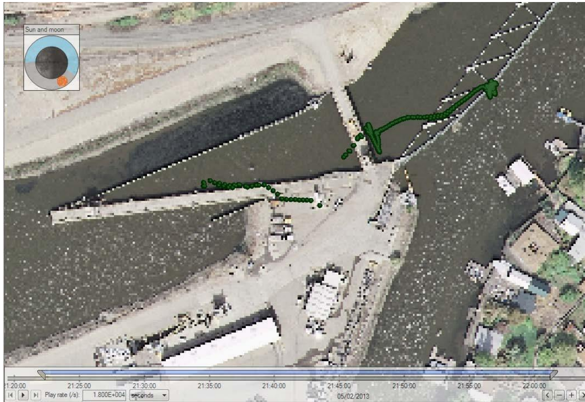
Figure C-34. Track of steelhead 2455 (released at high flow, total time in system was about 2 h: 2 min in the upstream channel, 2 min along the trash rack, 1 min in the primary channel, and almost 2 h in the bypass pipes/secondary channel).
