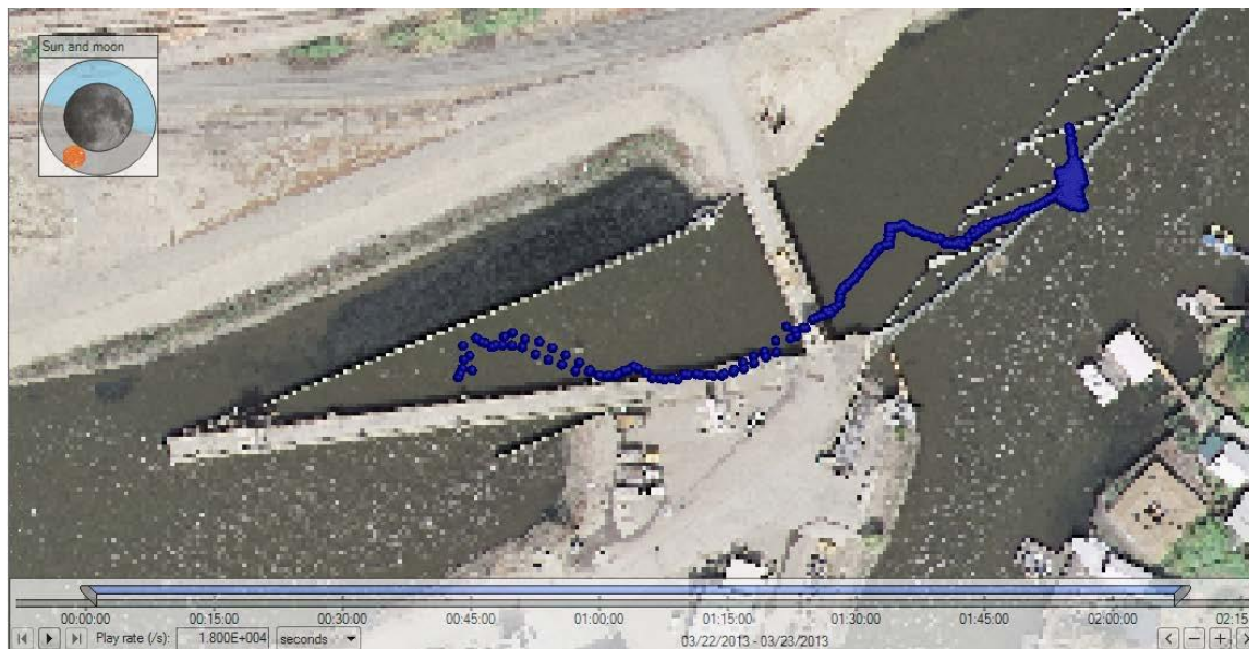
Figure C-5. Track of Chinook salmon 2119 (released at intermediate flow, total time in system was about 7 min: spent about 2.5 min in the upstream channel, < 1 min along the upstream side of the trash rack, 1 min in the primary channel and 3 min moving through the bypass pipes/secondary channel).
