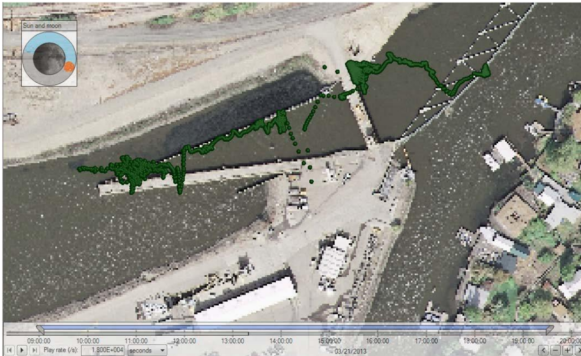
Figure C-30. Track of steelhead 2063 (released at high flow, total time in system was over 24 h: just over 1 h in the upstream channel, over 7 h in the primary channel and about 16 h in the bypass pipes/secondary channel).
