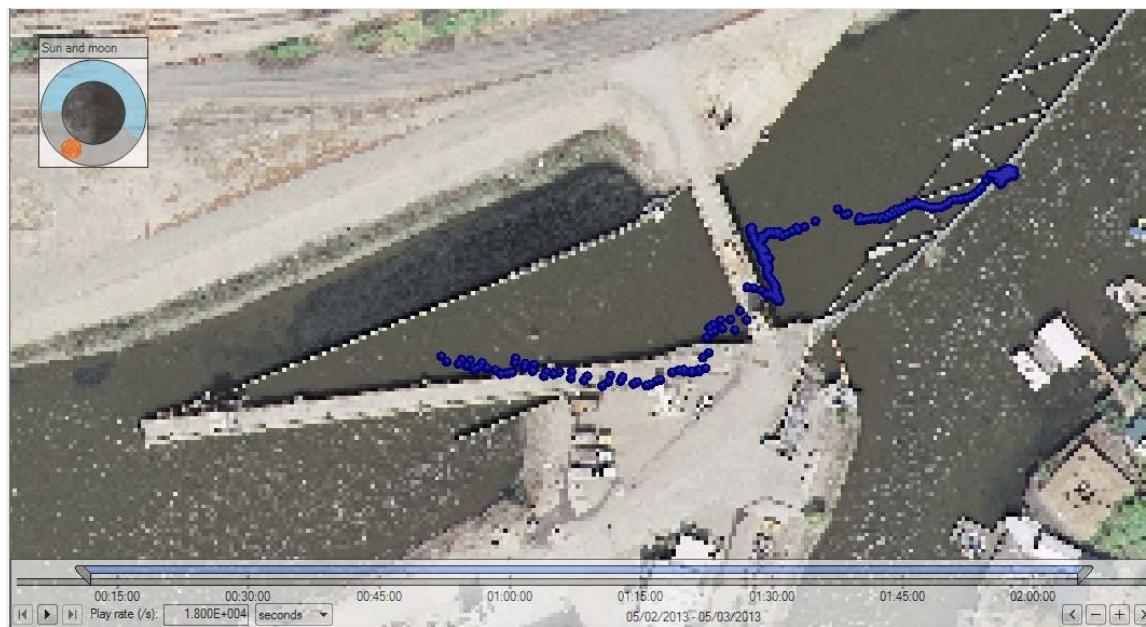
Figure C-17. Track of Chinook salmon 2231 (released at high flow, total time in system was about 9 min: 3 min in the upstream channel, 3 min along the trash rack, and 3 min through the primary channel/bypass pipes/secondary channel into the holding tank).
