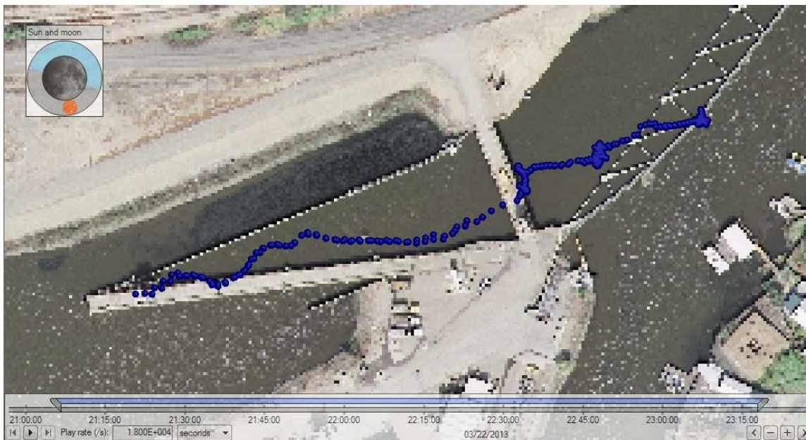
Figure C-11. Track of Chinook salmon 3883 (released at intermediate flow, total time in system was about 18 min: about 9 min in upstream channel, 2.4 min along the trash rack, 3.3 min in the primary channel, and 3.5 min moving through the bypass pipes and secondary channel).
