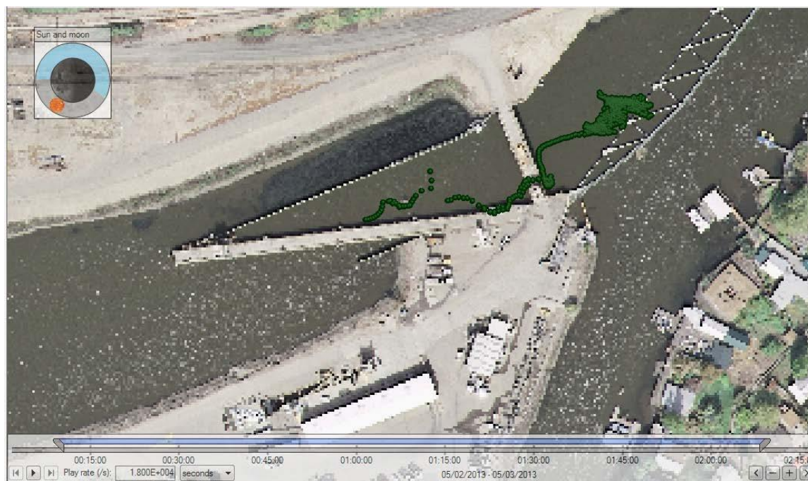
Figure C-35. Track of steelhead 2763 (released at high flow, total time in system was 0.6 h: 2 min in the upstream channel, 3 min along the trash rack, 2 min in the primary channel, and 28 min in the bypass pipes/secondary channel).
