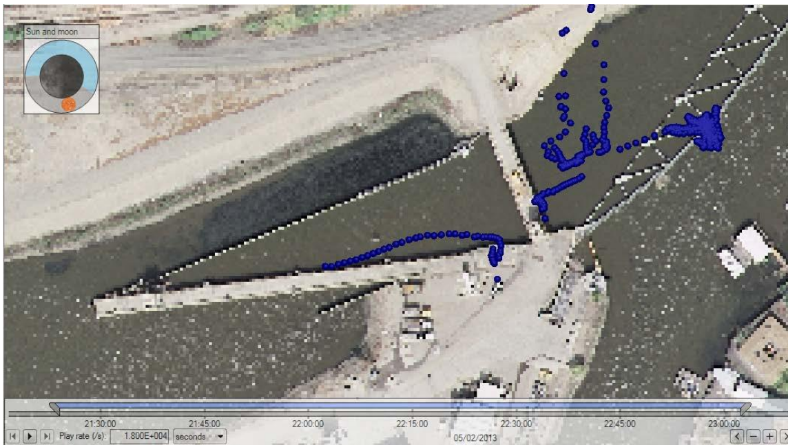
Figure C-23. Track of Chinook salmon 3267 (released at high flow, total time in system was about 29 min: 3 min in the upstream channel, 1 min along the trash rack, 1 min through the primary channel, and 25 min in the bypass pipes/secondary channel).
