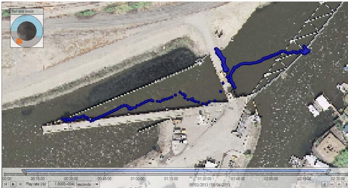
Figure C-6. Track of Chinook salmon 2623 (released at intermediate flow, total time in system was about 31 min: spent 2 min moving toward the trash rack, about 23 min moving along upstream side of the trash rack, 3 min in the primary channel, and 3 min moving through the bypass pipes/secondary channel).
