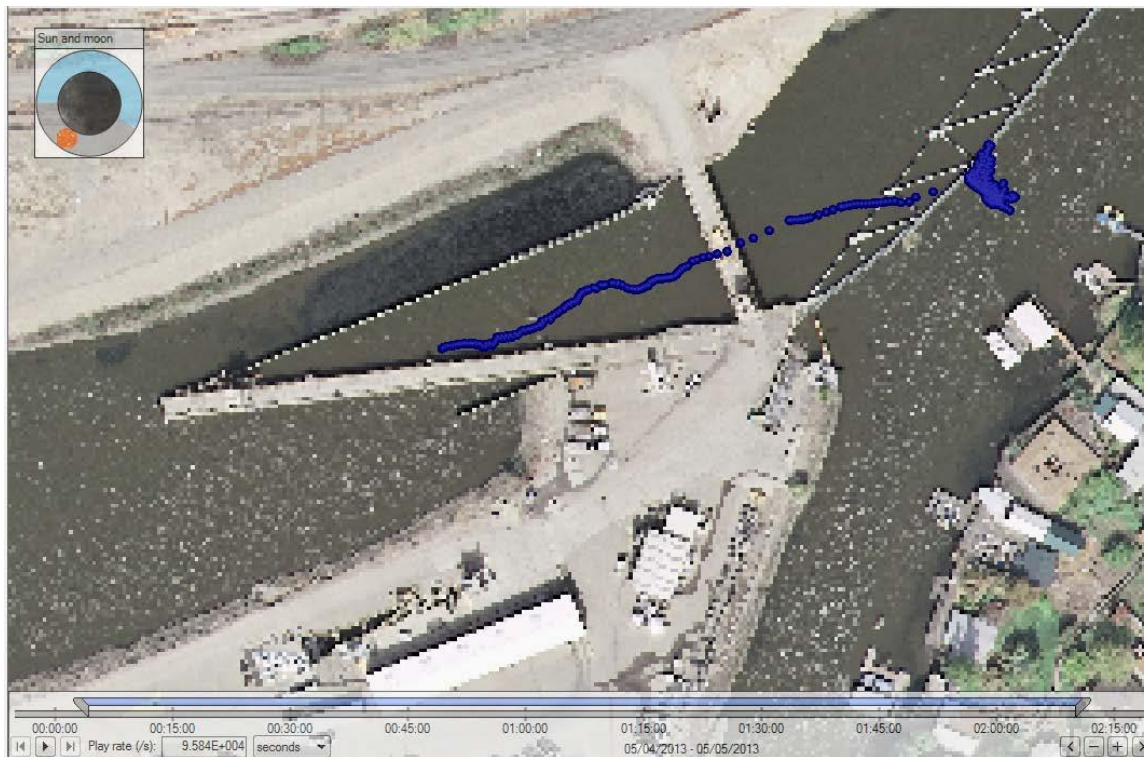
Figure C-3. Track of Chinook salmon 3239 (released at low flow, total time in system was 12 min: spent about 4 min in the upstream channel, < 1 min along upstream side of trash rack, 6 min in the primary channel, and 2 min in the bypass pipes/secondary channel).
