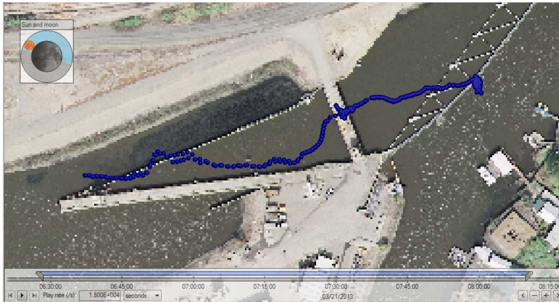
Figure C-20. Track of Chinook salmon 2847 (released at high flow, total time in system was about 12 min: 5 min in the upstream channel, 2 min along the trash rack, 3 min in the primary channel and 2 min through the bypass pipes/secondary channel to the holding tank).
