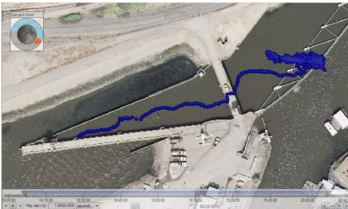
Figure C-7. Track of Chinook salmon 2735 (released at intermediate flow, total time in system was about 7 min: 2 min in the upstream channel, < 1 min along upstream side of the trash rack, 3 min in the primary channel, and 2 min in the bypass pipes/secondary channel).
