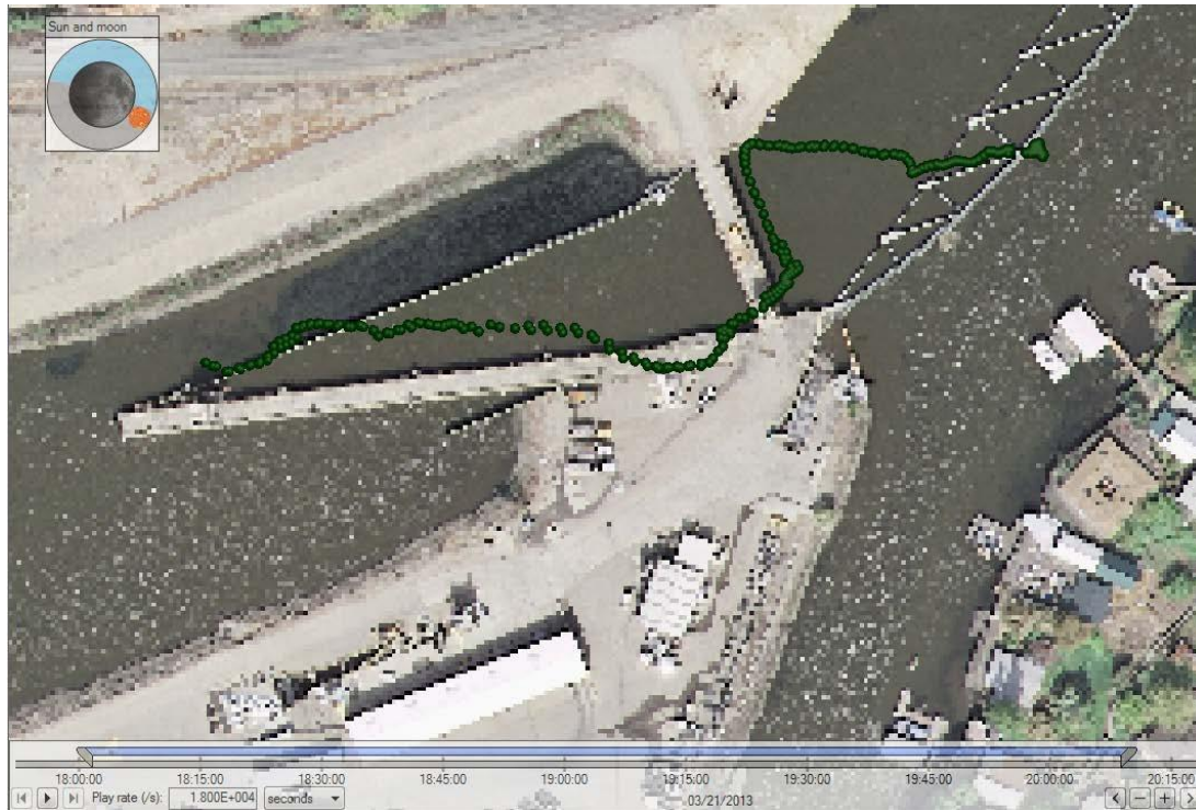
Figure C-32. Track of steelhead 3211 (released at high flow, total time in system was over 11 h: 4 min in the upstream channel, 1.5 min along the trash rack, 3 min through the primary channel, and over 11 h in the bypass pipes/secondary channel).
