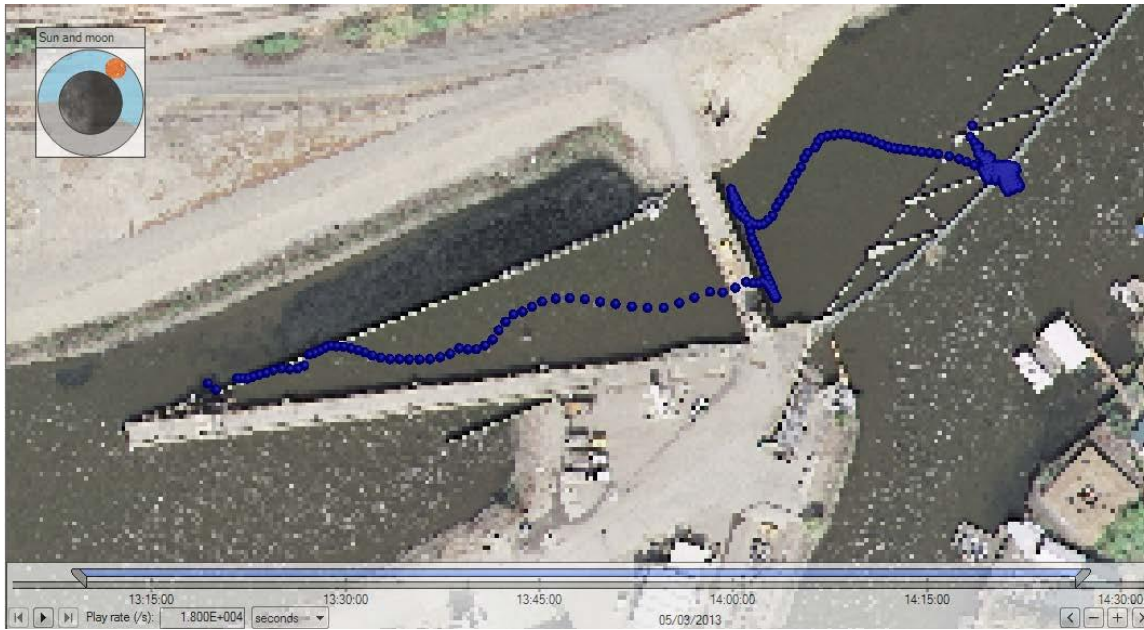
Figure C-12. Track of Chinook salmon 3939 (released at intermediate flow, total time in system was about 29 min: 3 min in the upstream channel, 3 min along the trash rack, 4 min in the primary channel, and 19 min in the bypass pipes/secondary channel).
