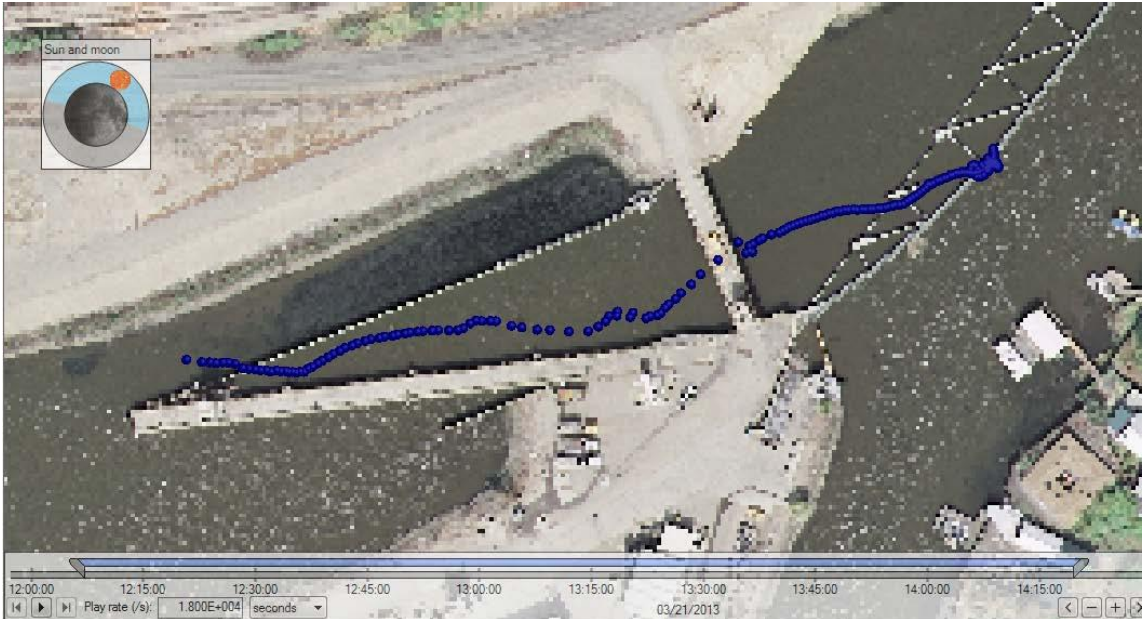
Figure C-25. Track of Chinook salmon 3323 (released at high flow, total time in system was about 7 min: 2 min in the upstream channel, < 1 min along upstream side of trash rack, 2 min through the primary channel, and 2 min in the bypass pipes/secondary channel).
