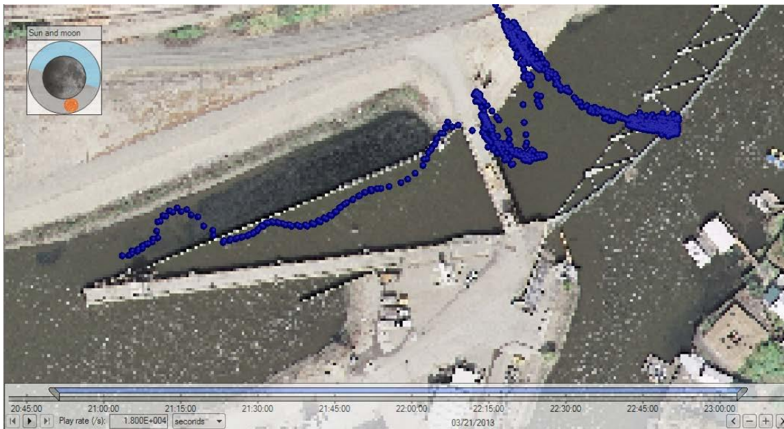
Figure C-15. Track of Chinook salmon 2007 (released at high flow, total time in system was about 41 min: 2 min in upstream channel and along the trash rack, 2 min in the primary channel, and 36 min in the bypass pipes/secondary channel before moving into a holding tank).
