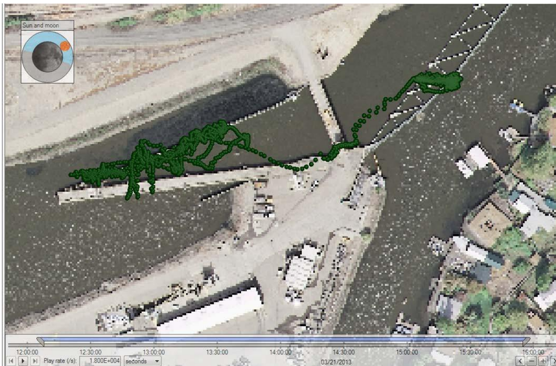
Figure C-31. Track of steelhead 3407 (released at high flow, total time in system was about 2.5 h: 3 min in the upstream channel, 1 min along the trash rack, over 1 h in the primary channel, and almost 1 h in the bypass pipes/secondary channel).
