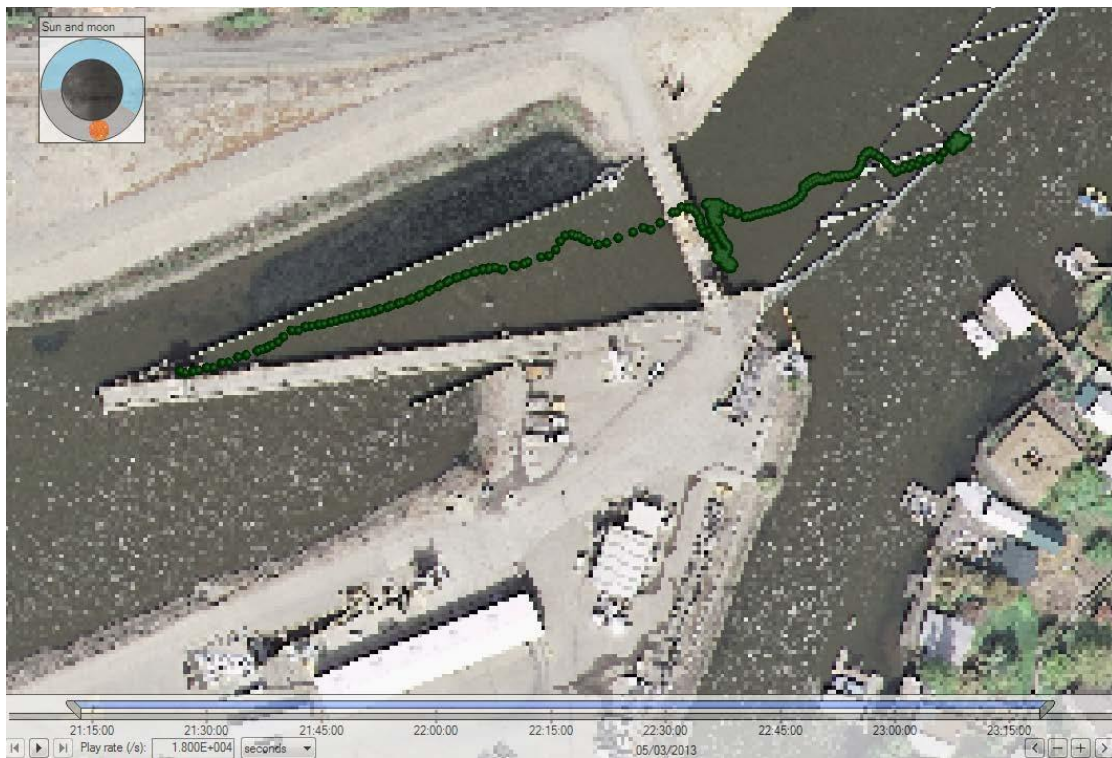
Figure C-29. Track of steelhead 3883 (released at intermediate flow, total time in system was 20 min: 3 min in the upstream channel, 10 min along the trash rack, 3 min in the primary channel, and 4 min in the bypass pipes/secondary channel).
