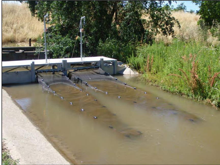
Figure 12. Two fyke nets, sampling platform, and associated apparatus used to sample for fish entrainment in the Tisdale canal.
