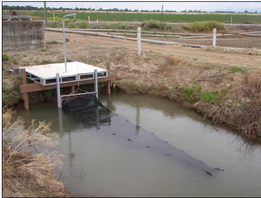
Figure 10. The fyke net, sampling platform, and associated apparatus used to sample for fish entrainment in the Townsite north canal.
