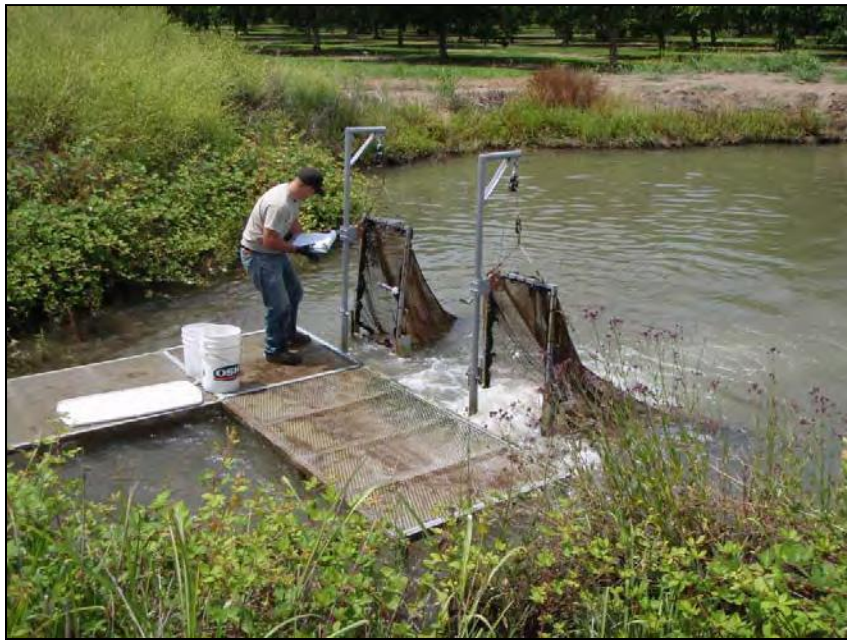
Figure 2. Fyke apparatus and nets used to sample for fish entrainment at the Sycamore canal.
