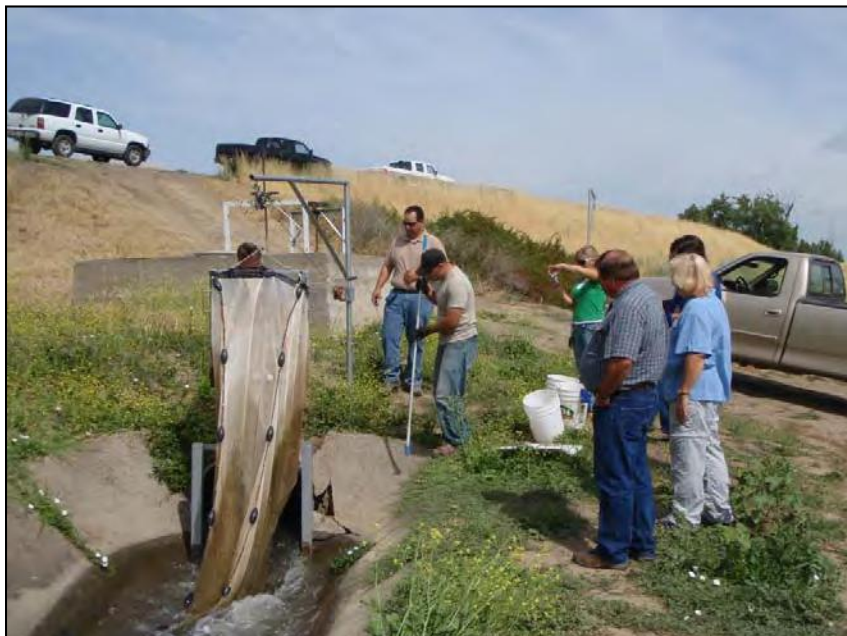
Figure 3. Fyke apparatus and net used to sample for fish entrainment in one of two canals at River Garden Farms No. 2.
