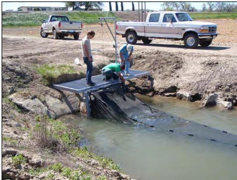
Figure 4. Fyke apparatus, fyke net, and sampling platform used to sample for fish entrainment in the State Ranch canal.
