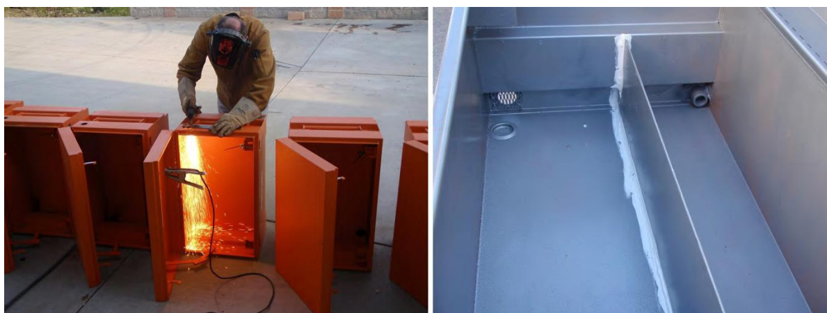
Figure 5. Modifications to the acoustic receiver boxes for the 2009 VAMP study. Left picture: plasma cutting ventilation holes. Right picture: inside of the modified job box showing the water bath compartment and drainage pipe on the right and the dry compartment on the left for housing the data logger and ventilation hole.
