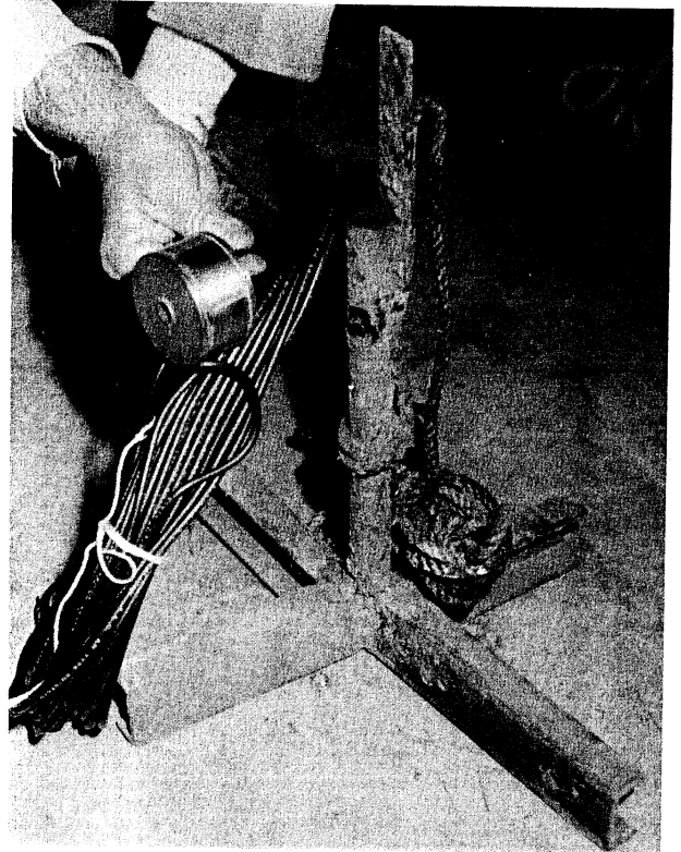
FIGURE 11. Hydrophone, iron stand used to hold it above the river bottom and lead-in cable. Photograph by Wm. F. Van Woert.
