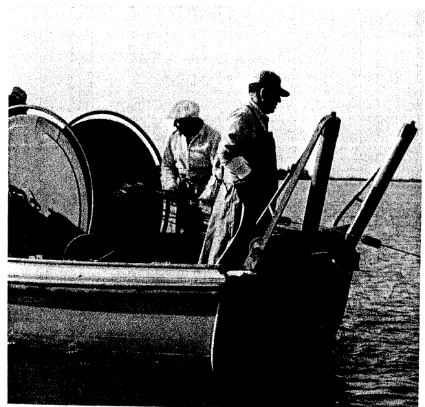
FIGURE 14. Trammel net being wound onto powered net reel on the M.V. Striper , San Joaquin River at Prisoners Point, fall, 1965. Photograph by Richard J. Hallock.
