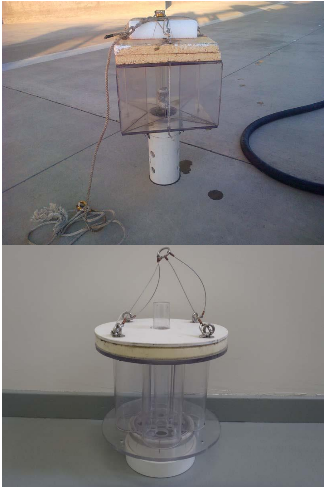
Figure 3. Two Types of Floating Larval Light Traps Used at the Freeport Water Intake Facility
