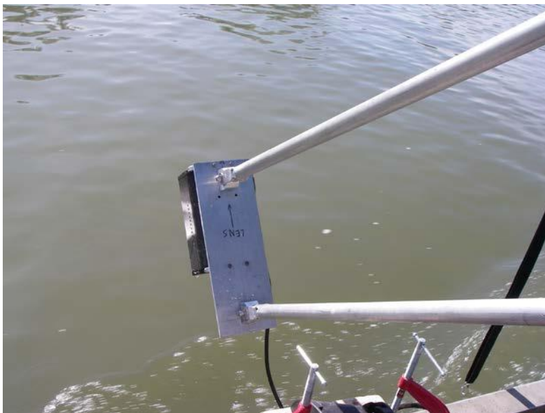
Figure 6. Pole Mount for Mobile Surveys using DIDSON/ARIS Sonar Camera
