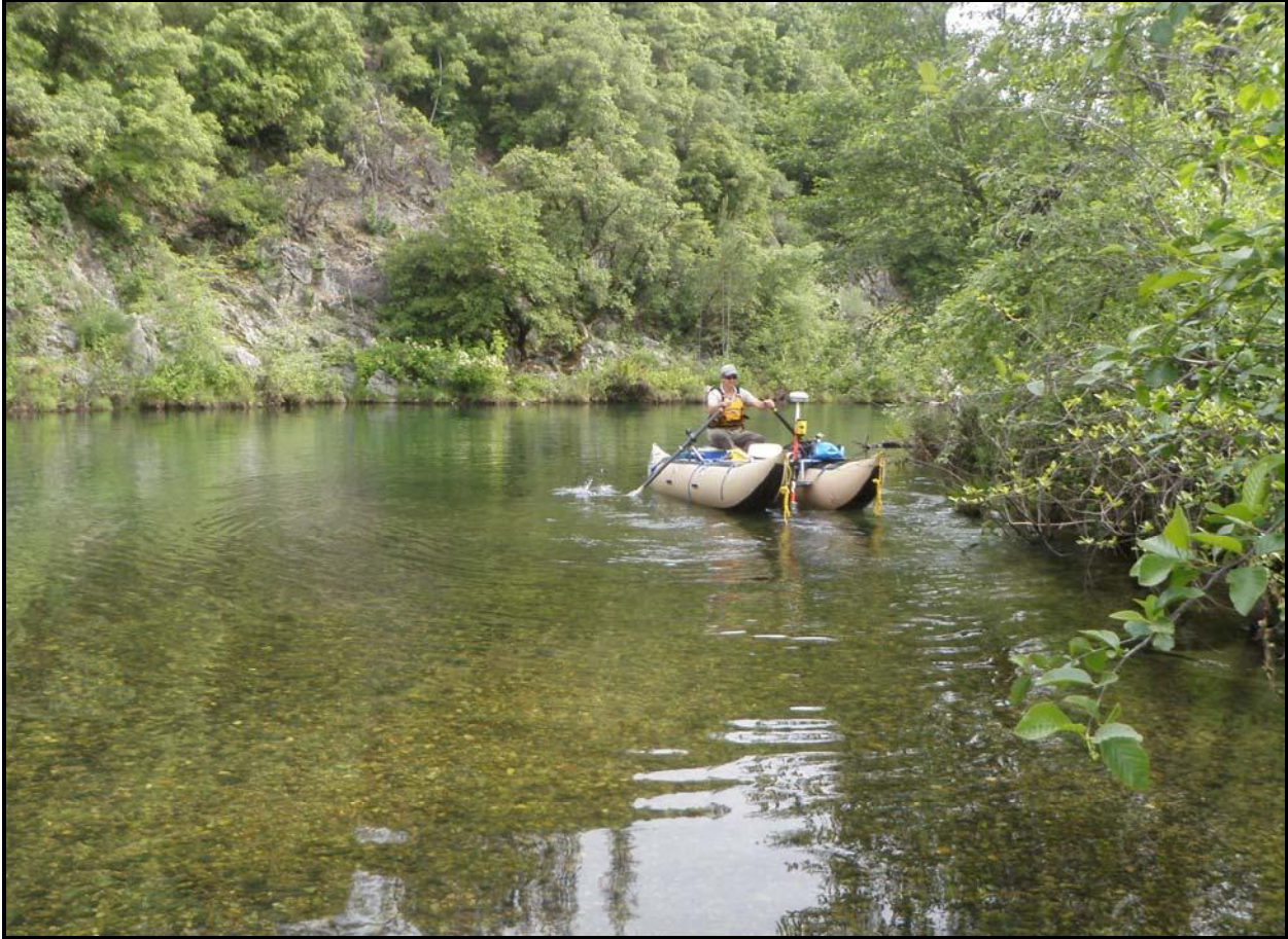
Figure 4. Cataraft-based survey platform utilizing depth sounder integrated with GPS-RTK system – shown here mapping the leading edge of the Whiskeytown gravel injection in “Pool 3.”
